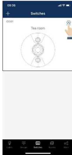
1. Select the setting button to configure the ceiling sensor.
