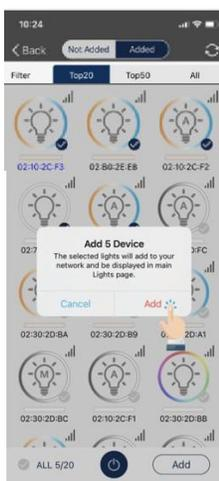
6. Confirm by selecting the “Add” button in the dialog box. A light will blink to indicate a successful connection.
