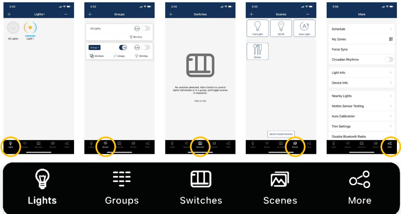
**"Lights"** shows all lights that are connected to the app. It allows the user to view and control individual lights.
