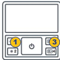
Press the **button 1 and 3** together and hold for 2 seconds and then release.
