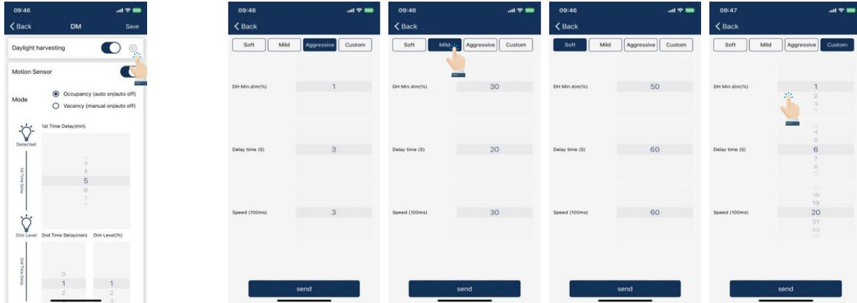
1. Select the setting button beside Daylight harvesting toggle button to set daylight harvesting
