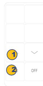
Press the **button 1 and 2** together and hold for 2 seconds and then release.
