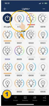
1. On the Lights page, select and hold a light icon to access the “Light Dimming” settings.
