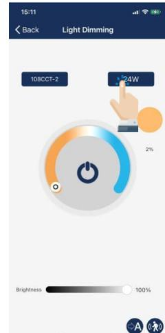
5. Note that the wattage is the rated wattage after High-Trim is set. E.g., input 24 for a 30-watt luminaire with 80% of High-End trim setting.
