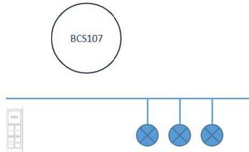
To provide vacancy and bi-level dimming on Keiltoninterior light together with the BCS107 ceiling sensor:
