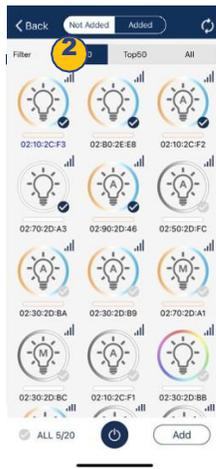
2. Select **Top20**, **Top50** or **All** from the filter at top of screen to show lights with the strongest Bluetooth signal
