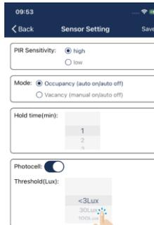
3. You may set the hold time of the PIR sensor, enable/disable photocell and set the photocell threshold.
