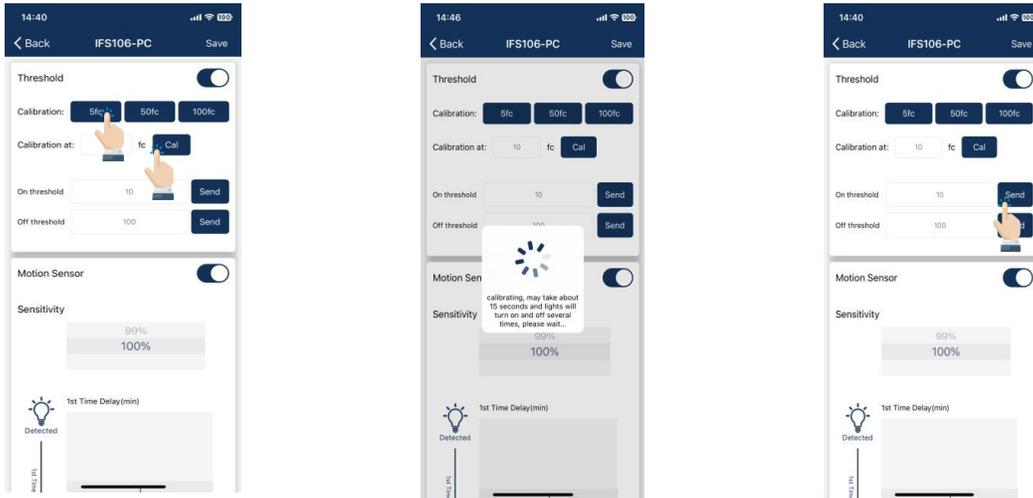
1. For photocell sensors, the default ON/OFF threshold is 10/60 fc. User may change the thresholds. Click the button of 5fc/50fc/100fc will set 5/50/100 fc as ON threshold respectively and the lights will turn on/off several times to auto-calculate the OFF threshold. User may input a specified fc value as ON threshold and select the “Cal” button to calculate the OFF threshold based on it.
