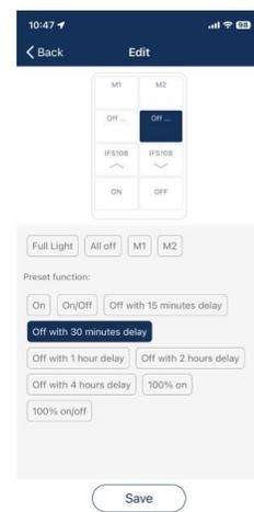
*Note: the timed off will be interrupted and canceled if user manually dims the lights, for example, turn on, manually dim up/down by APP, switch or schedule.*
