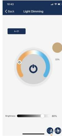
2. Adjust the dimming levels and color temperature as desired.
