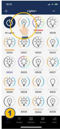
1. From the Lights page, do an extended press and hold on a light's icon to open the Light Dimming settings page.
