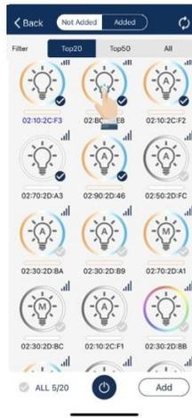
3. The APP will scan for lights that can be added to the zone. Lights can be identified in a room by pressing the icons to turn it on and off.
