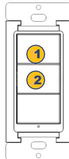
Press the **button 1 and 2** together and hold for 2 seconds and then release.
