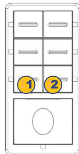
Press the **button 1 and 2** together and hold for 2 seconds and then release.
