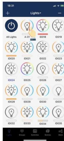
3. Lightly slide a finger up or down over a light's icon to adjust the color temperature.
