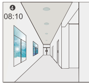
When the natural light level exceeds setpoint off to light, the light will turn off even if when the space is occupied.
